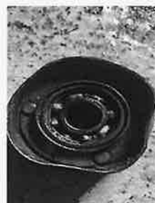
Figure 3: Suspected tensioner bearing problem
