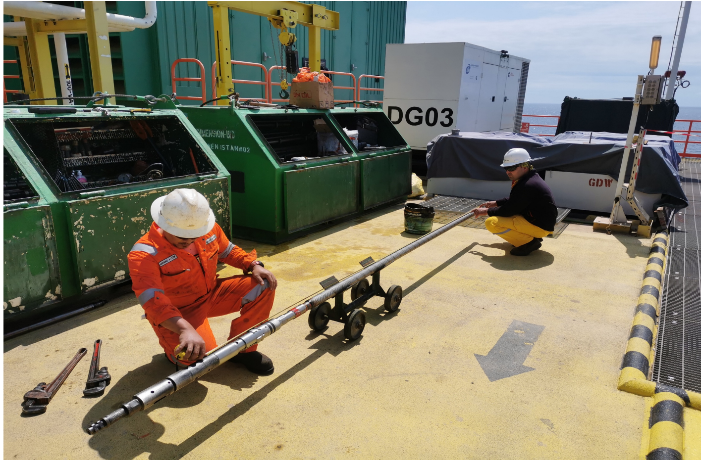
Fig 6 : Measure the TTSS with XN-lock mandrel
