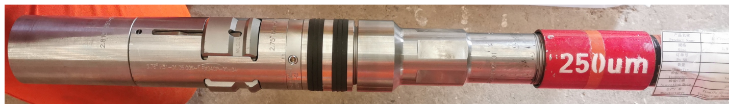
Fig 4 : Lock Mandrel with 250 microns TTSS
