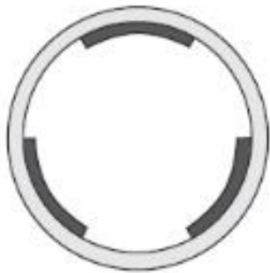
Conventional Pulling Tool 50 % Contact Area
