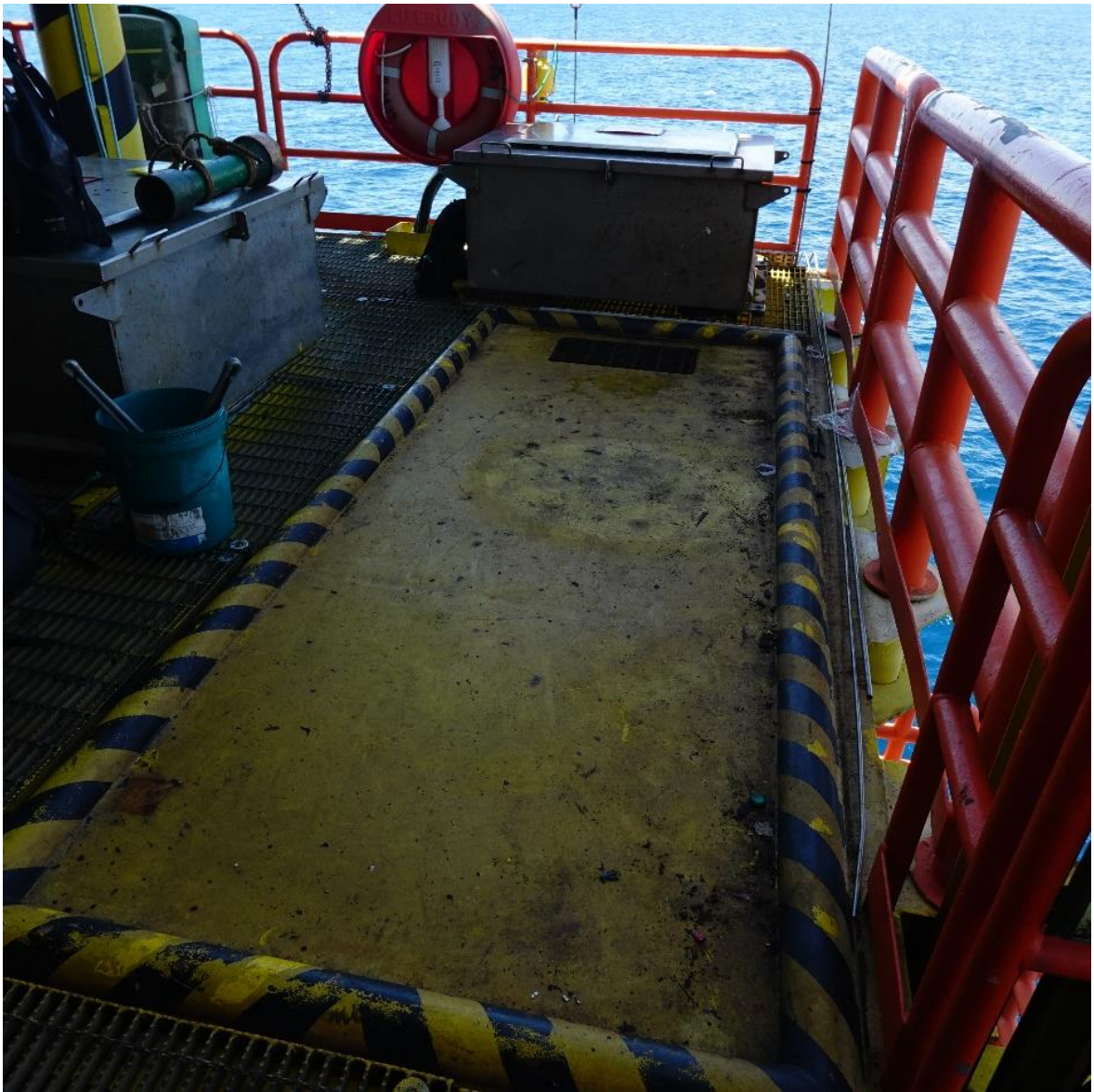
Fig: Loading Bay on Cellar Deck, In Front of Control Room. Usable Area 12 ft x 4 ft.
