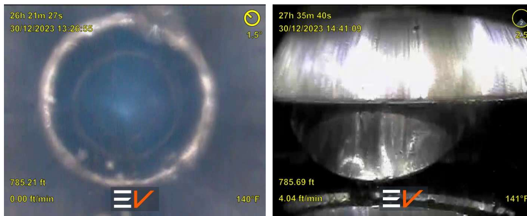
Fig.1.1 EGF Flapper condition at 786 ft
