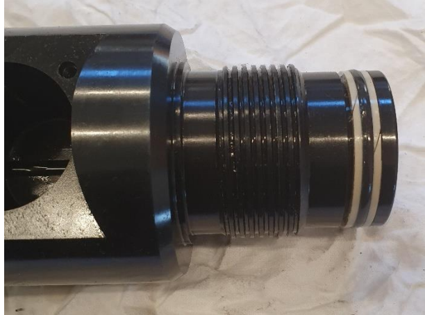
Figure 50 - Seal arrangement fitted to Punch Housing image
