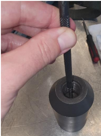
Figure 122 - Pin Punch through the End Sub to remove the Relief Piston image
