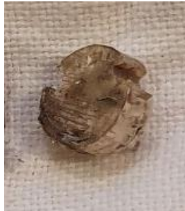
Figure 121 - Circular Relief Shear Disc fragment
