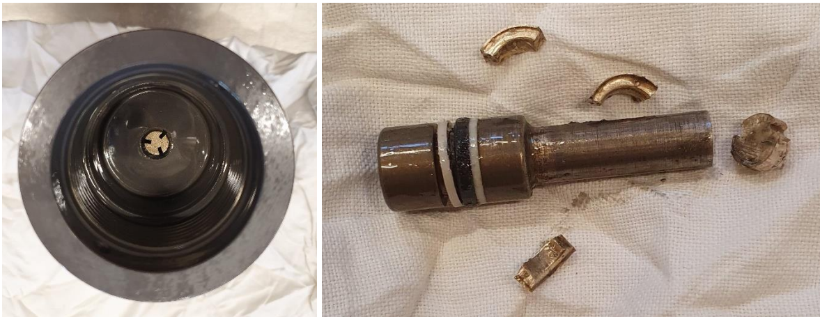
Figure 14 - Relief Disc image fitted into End Sub and remnants of the sheared Disc after deployment
