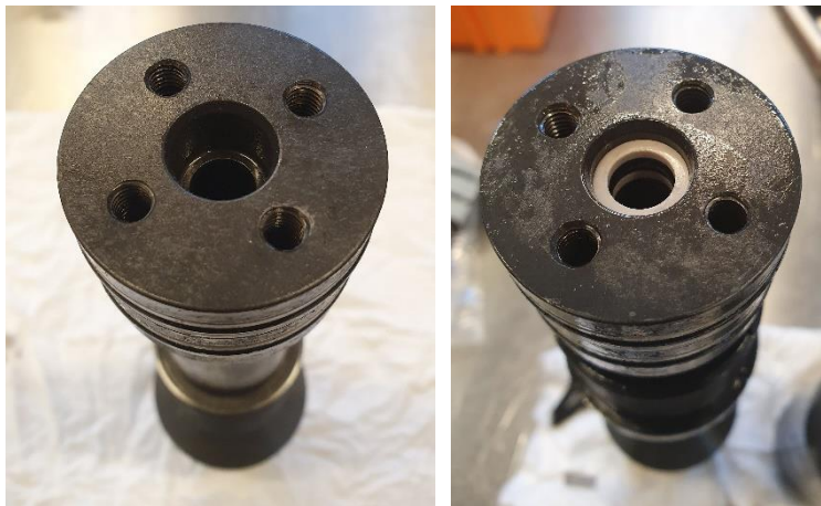
Figure 26 – Tubing Nipple sealing arrangement location and fitment images
