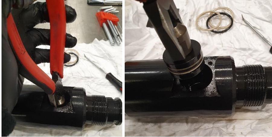
Figure 126 - Punch Piston removal images
