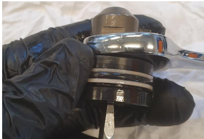
Figure 127 - Punch Holder removal image
