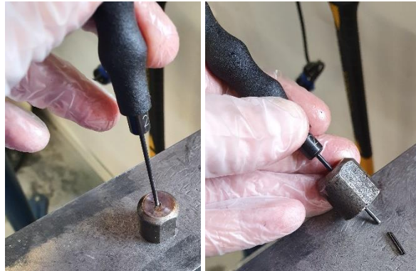
Figure 128 - Spring Pin removal images
