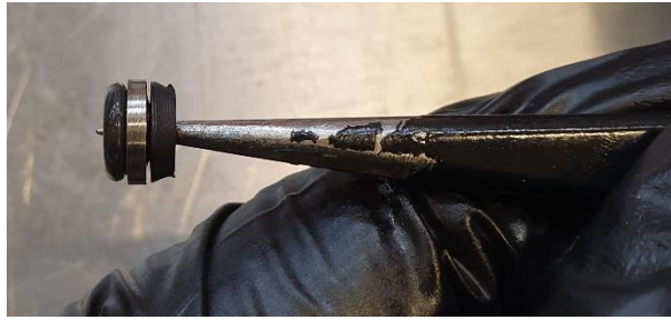
Figure 39 - Check Valve Seal and O-Ring fitted to Insert
