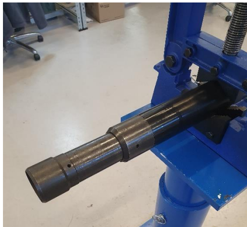
Figure 38 - Extension Sub assembly fitted to the Piston Housing
