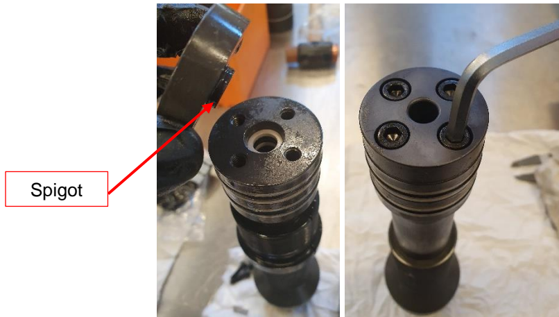
Figure 27 – End Plate orientation and installation image
