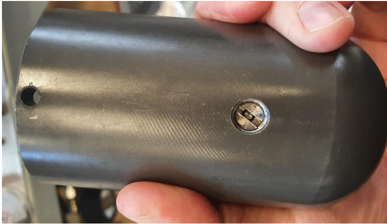
Figure 42 - Image showing Check Valve assembly fitted
