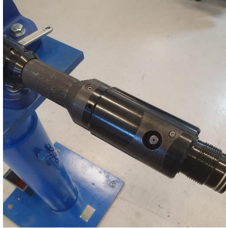
Figure 57 - Punch Head fitted to Hydraulic Actuator
