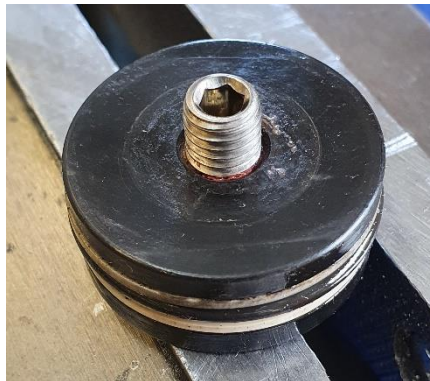
Figure 51 - Set Screw fitted to Punch Piston
