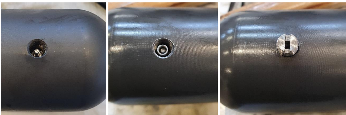
Figure 41 - Images Showing Check Valve, Spring and Check Valve Housing Fitment
