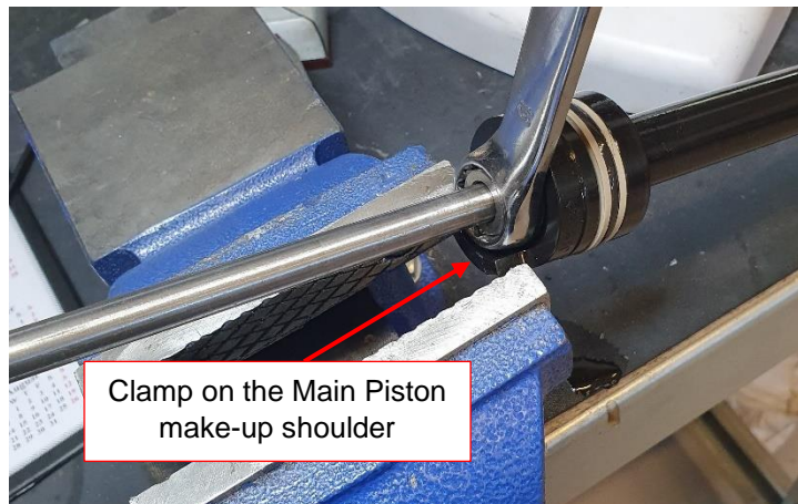
Figure 32 - Make-up of Tubing Nipple to Main Piston
