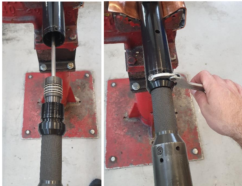
Figure 34 - Outlet Sub installation
