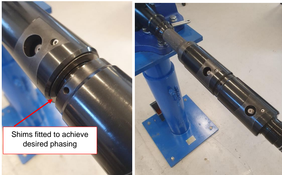
Figure 59 - Punch Head phasing images. The above example has been shimmed for 0° phasing
