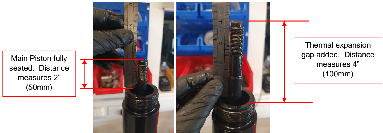
Figure 65 - Images showing the fully seated position on the left (2"), and the position once the thermal expansion gap has been inserted (4")
