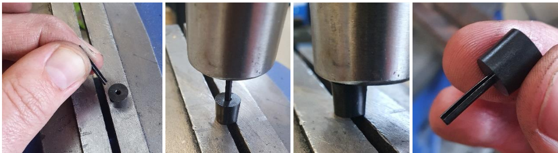
Figure 80 - Spring Pin installation images
