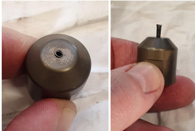
Figure 124 - Punch Holder with fragment of Spring Pin images
