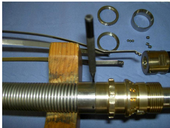
Figure C.4 Removal of the Spirol Pins from the Spring Retaining Ring
