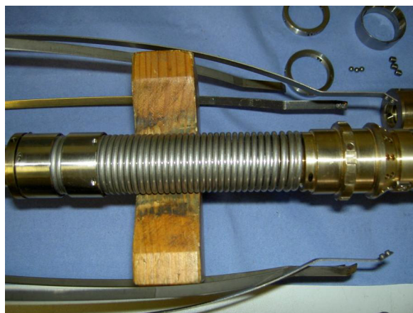
Figure C.8 Extension Spring and the Restrictor Ring installed over the Main Shaft
