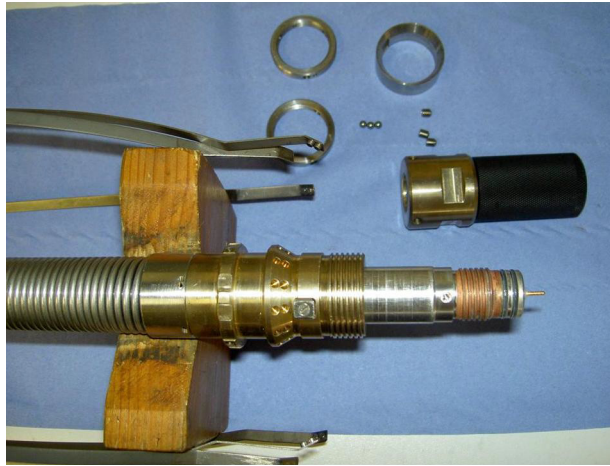
Figure C.3 Locking Rings, Clamp Ring and Springbows removed from the Lower End Termination Body
