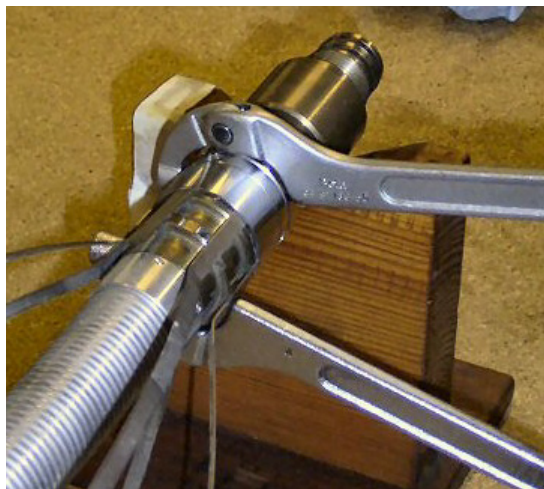
Figure 5.2 Loosen the Bow Clamp Locking Rings
