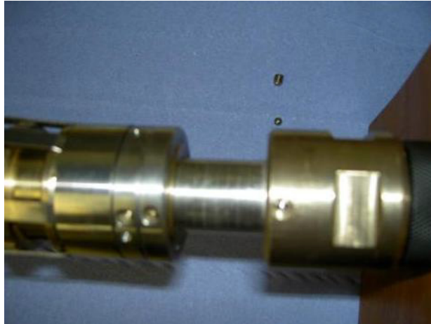
Figure C.9 Lower End Clamp Ring held in position by the two Bow Clamp Locking Rings
