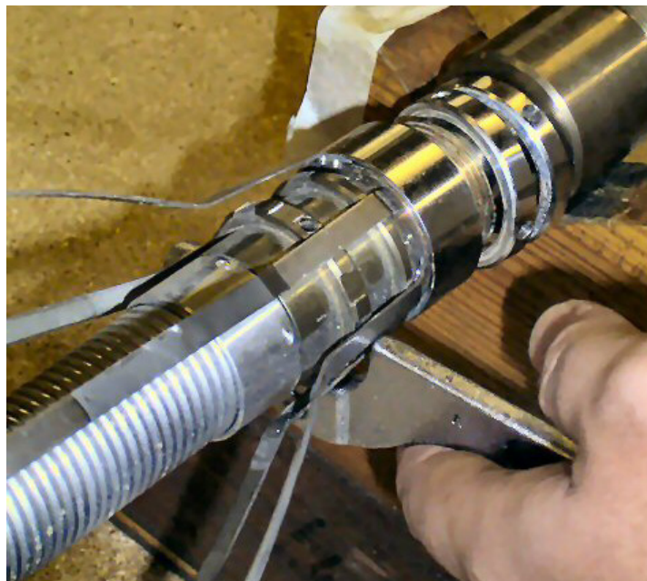
Figure 5.4 Loosening the Bow Clamp Split Rings
