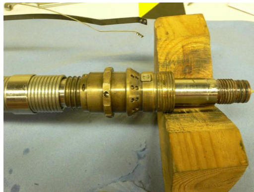
Figure C.5 Lower End Termination Body removed
