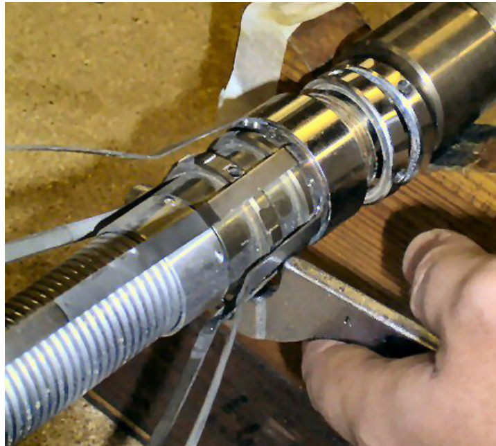
Figure 5.13 Installation of the Bow Clamp Outer ring and the Bursting Disc
