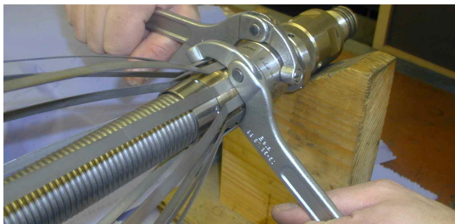
Figure 5.14 Tightening of the Bow Clamp Locking Rings
