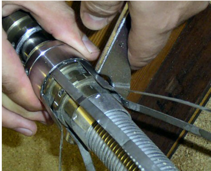
Figure 5.3 Sliding away the Lower Bow Clamp Ring
