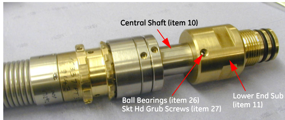
Figure 5.10 Lower End Sub screwed onto the Central Shaft
