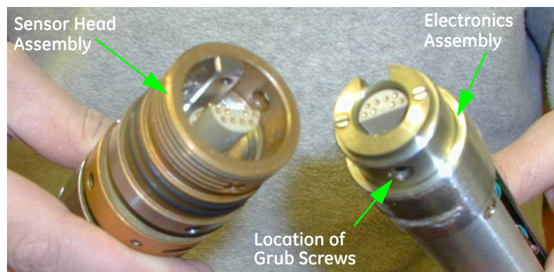
Figure 5.15 Connecting the Electronics Assembly to the Sensor Head Assembly
