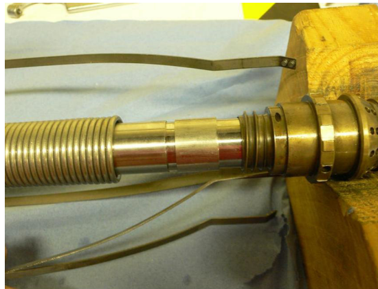
Figure C.7 Restrictor Ring installed
