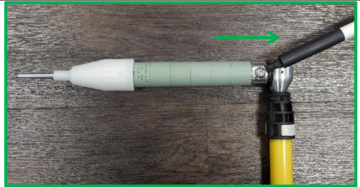
Tighten the HV cable to the discharge resistor. The cable must lie to the rear of the discharge resistor.
