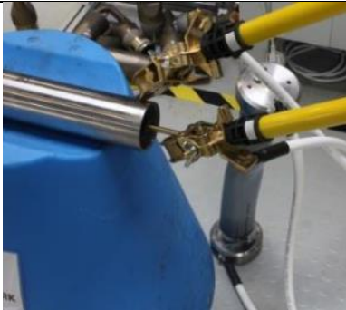
Use the sticks to short-circuit the PSU
