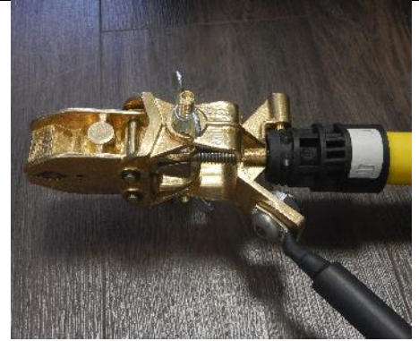
Tighten the HV cable (IA9690003000-B) to the ground clamp.
