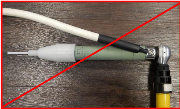
Tighten the HV cable to the discharge resistor. The cable must lie to the rear of the discharge resistor.
