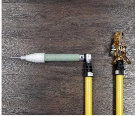
Insert the ground clamp (MP0000004000-A) and the discharge resistor (IA9190001000-A) in the sticks.
