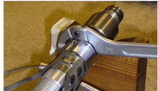
Figure 5.2 Loosen Bow Clamp Locking Rings
