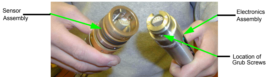
Figure 5.1 Separating Electronics from Sensor Head Assembly
