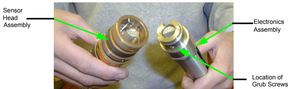
Figure 5.12 Connecting Electronics to Sensor Head
