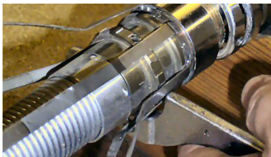
Figure 5.4 Loosening Bow Clamp Split Rings
