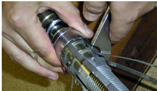
Figure 5.3 Sliding lower bow clamp ring away.
