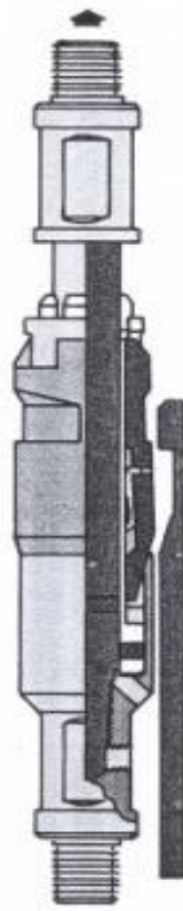
Keys retracted when pin sheared if SSD is too tight.
