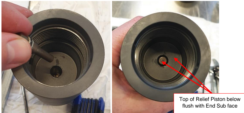
Figure 49 - Relief Piston fitment images
