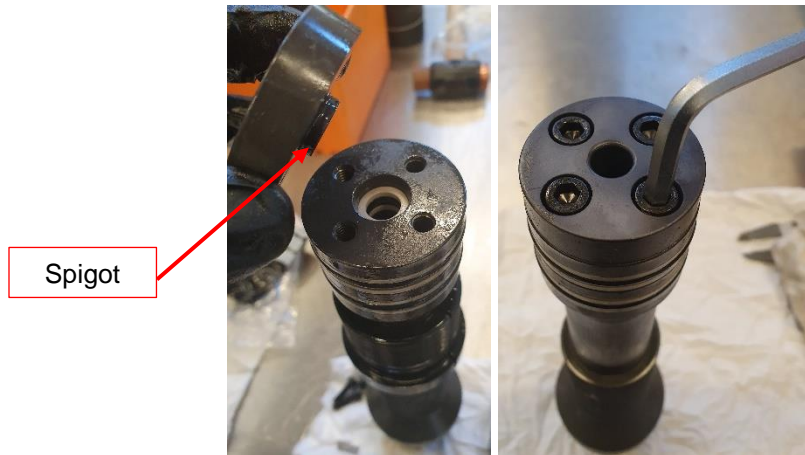
Figure 28 – End Plate orientation and installation image
