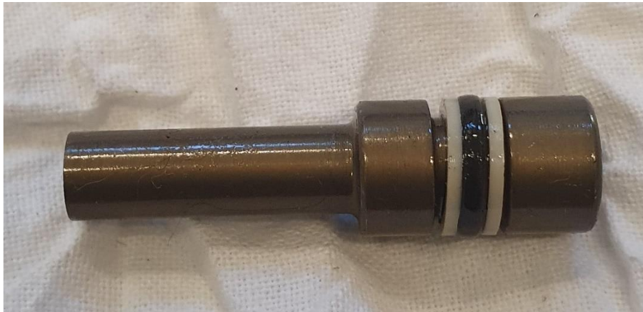
Figure 44 - Relief Piston seal arrangement image
