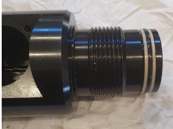
Figure 51 - Seal arrangement fitted to Punch Housing image
