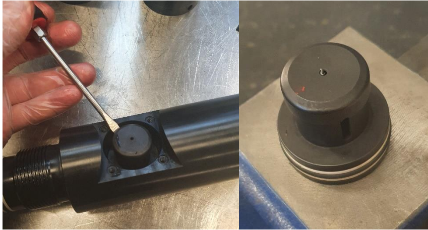
Figure 131 - Punch Piston removal images
