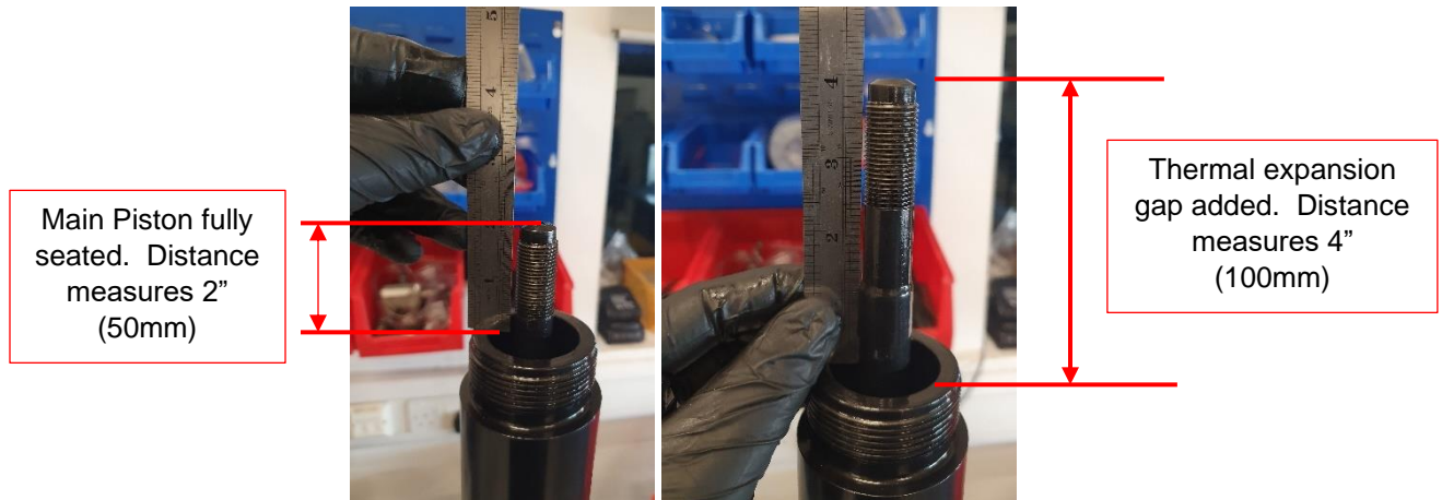
Figure 66 - Images showing the fully seated position on the left (2"), and the position once the thermal expansion gap has been inserted (4")
