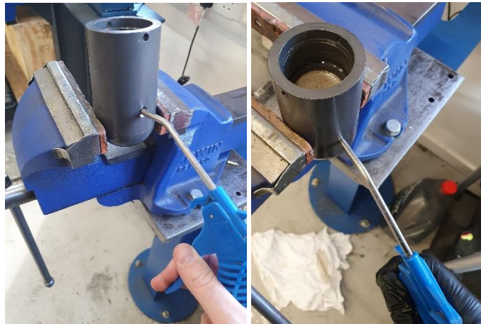
Figure 46 - Check Valve leak test images
