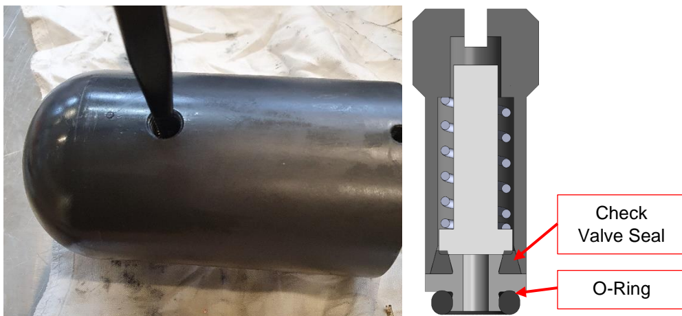
Figure 41 - Check Valve Insert Orientation image
