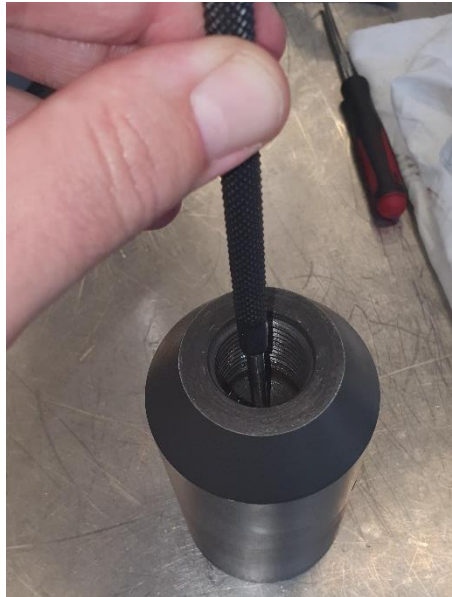
Figure 47 - Access hole to remove Relief Piston image
