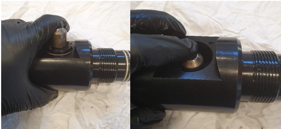
Figure 54 - Punch Piston installation image
