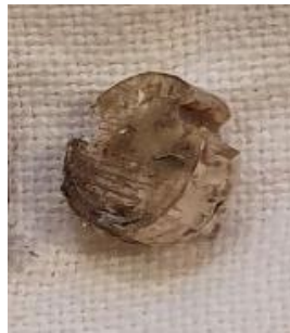
Figure 122 - Circular Relief Shear Disc fragment
