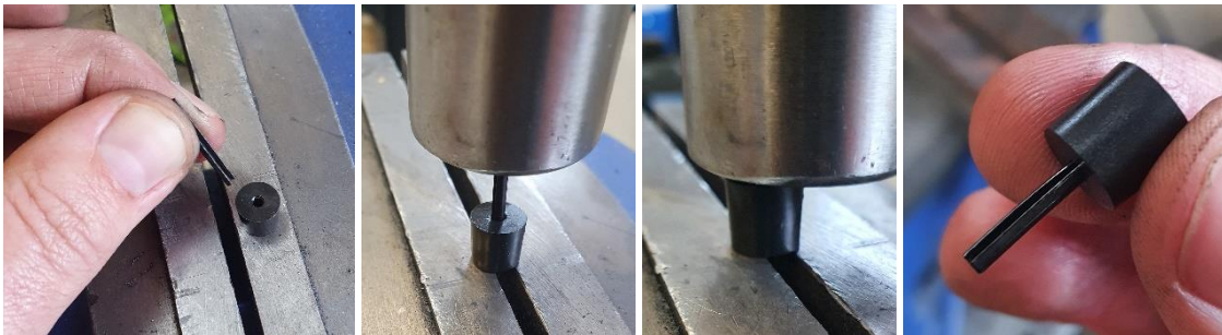
Figure 81 - Spring Pin installation images
