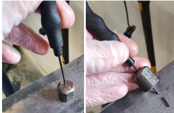
Figure 129 - Spring Pin removal images
