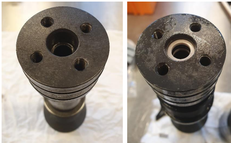
Figure 27 – Tubing Nipple sealing arrangement location and fitment images
