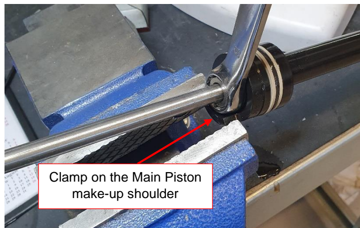
Figure 33 - Make-up of Tubing Nipple to Main Piston
