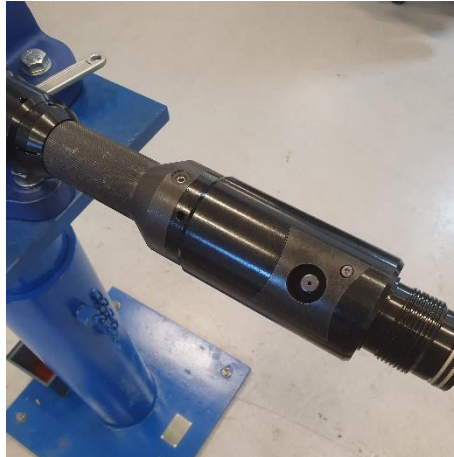
Figure 58 - Punch Head fitted to Hydraulic Actuator
