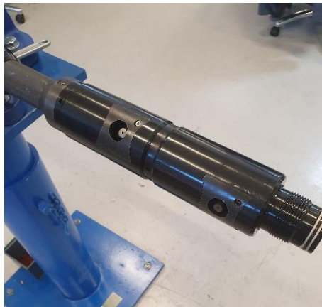
Figure 59 - Second Punch Head fitted
