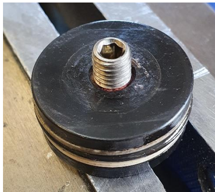
Figure 52 - Set Screw fitted to Punch Piston
