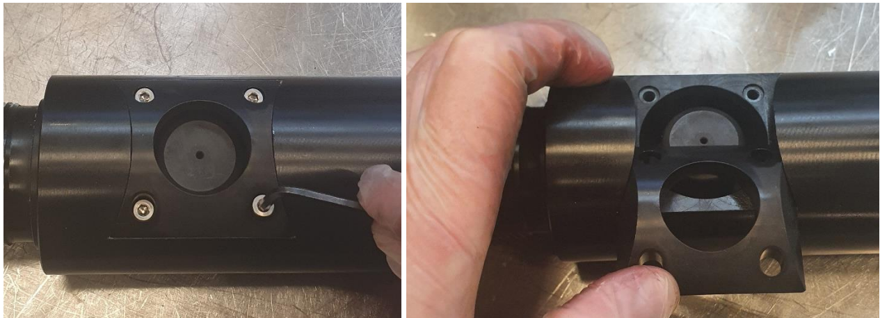
Figure 130 - Retainer Plate removal image
