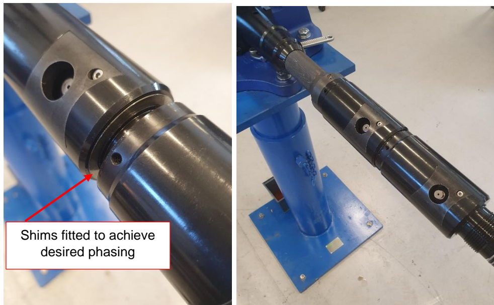
Figure 60 - Punch Head phasing images. The above example has been shimmed for 0° phasing
