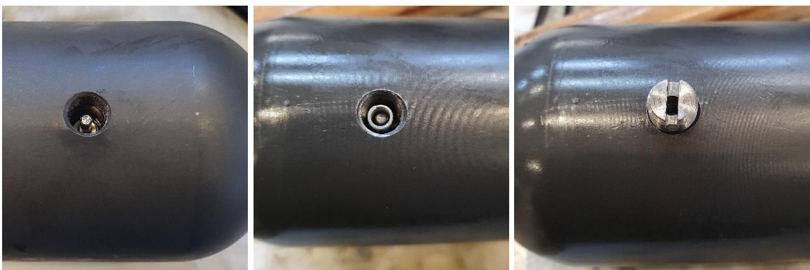
Figure 42 - Images Showing Check Valve, Spring and Check Valve Housing Fitment
