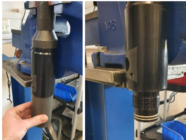
Figure 64 - End Sub removal image
