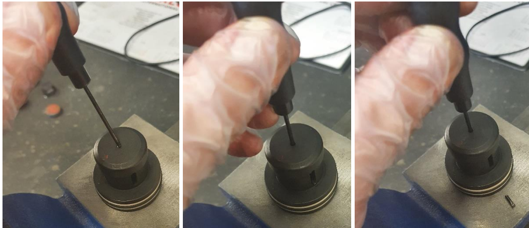
Figure 132 - Spring Pin removal images
