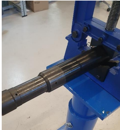
Figure 76 - Retainer Cap make-up image
