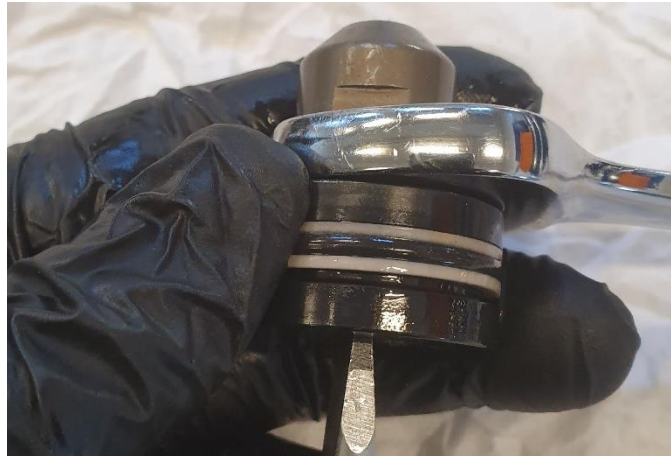
Figure 53 - Fitting of Punch Holder to Punch Piston image
