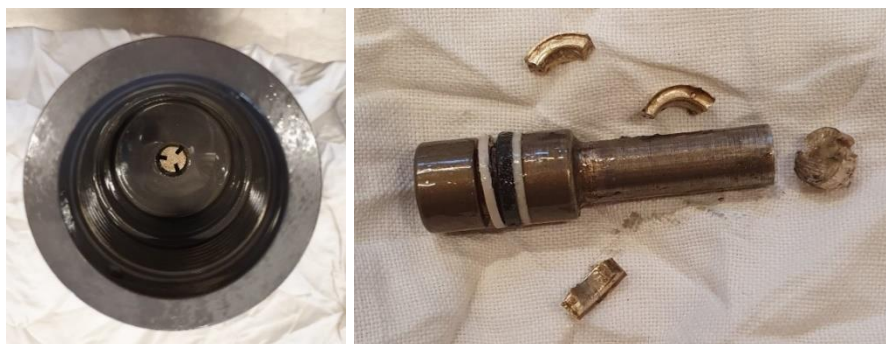
Figure 15 - Relief Disc image fitted into End Sub and remnants of the sheared Disc after deployment
