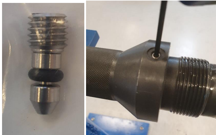
Figure 25 - A.F.O Plug image and assembly
