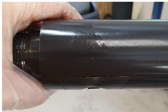
Figure 79 - When held upside down the Punch Button should remain secure
