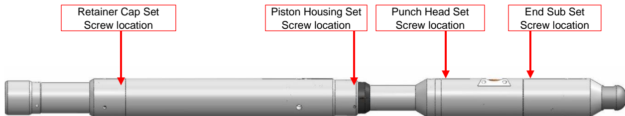
Figure 77 - Retaining Set Screw location image
