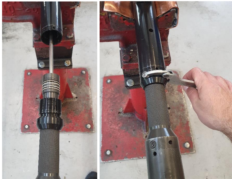
Figure 35 - Outlet Sub installation
