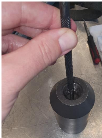
Figure 123 - Pin Punch through the End Sub to remove the Relief Piston image
