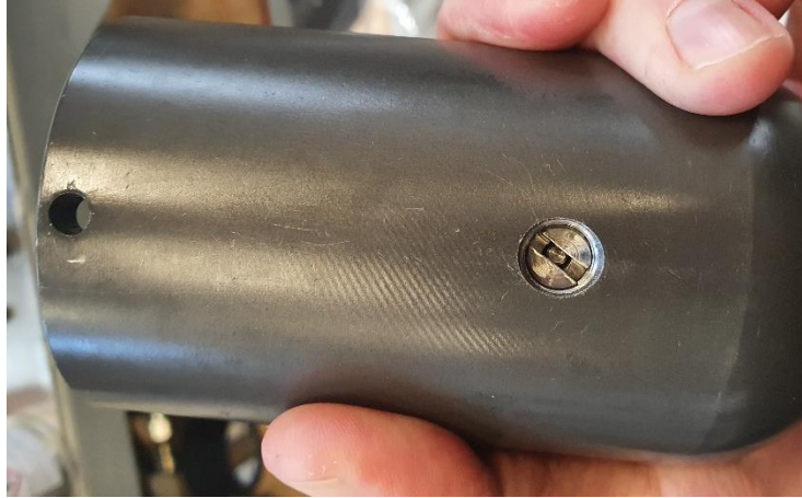
Figure 43 - Image showing Check Valve assembly fitted
