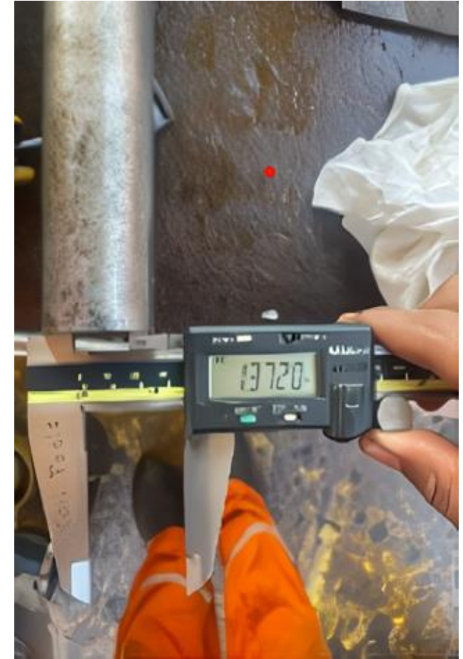
Figure 3 – ID of Packing mandrel = 1.372"
