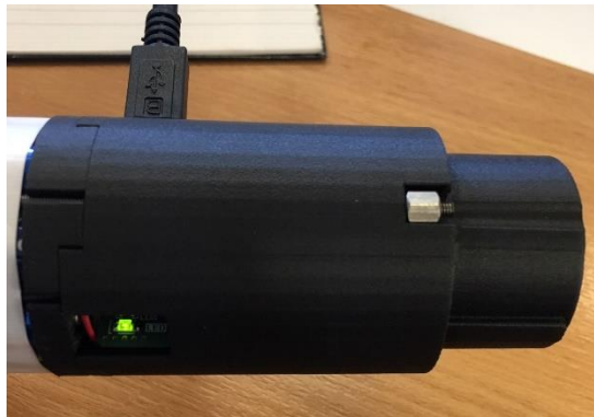
Figure 58 - USB connected to PCM and diagnostic LED illuminated
