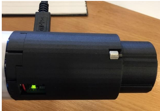
Figure 31 – Photo of PCM connected and LED diagnostic indicator
