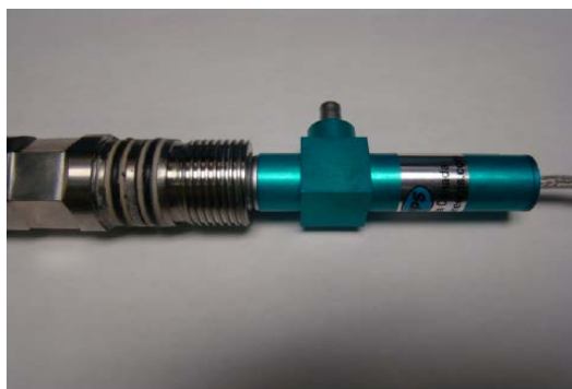
Figure 2. USB communication box connected to gauge
