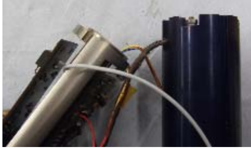
Figure 5-25 Rotate the Electronics Chassis from the Electronics Mount Sleeve
