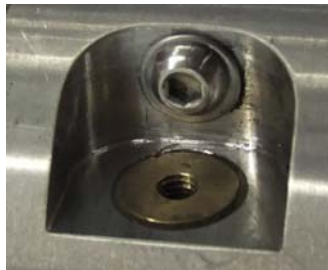
Figure 5-7 Remove the Grub Screw from the Pressure Relief Valve
