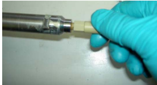
Figure 5-10 Remove the Lower Retaining Connector Nut
