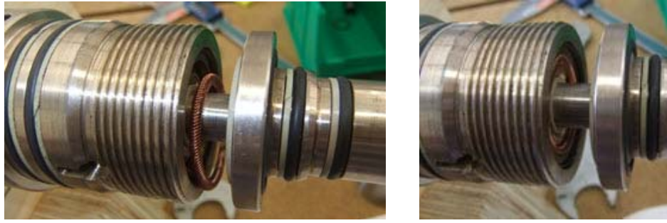
Figure 5-20 Insulating Washer, Canted Coil Spring and Seal Cartridge
