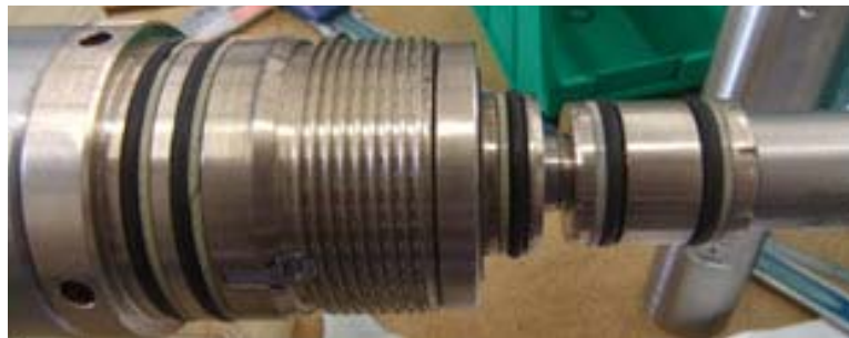
Figure 5-21 Fitting the Piston Shuttle Valve
