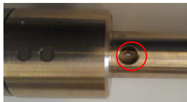
(Above) The Nipple Contact Insulator not aligned
