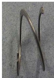
Figure 5-37 Strained Internal Spiral Retaining Ring
