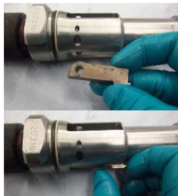
Figure 5-39 Alignment and fitment of the Latching Dogs
