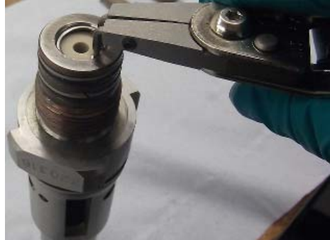
Figure 5-36 Remove the Circlip from the Bottom End of the Fishing Neck
