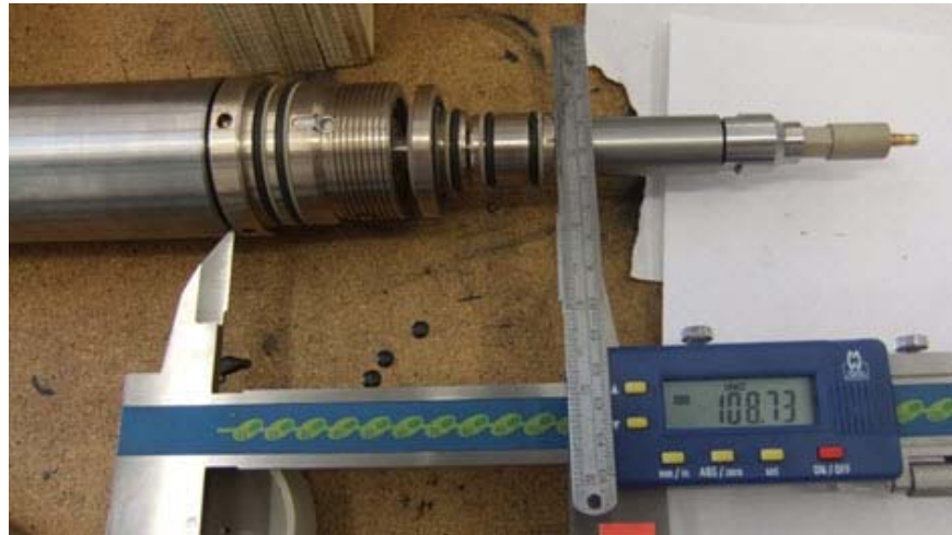
Figure 5-23 Measure the distance from the Joint to the Piston Shuttle Valve
