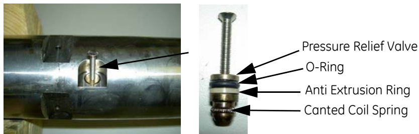
Figure 5-8 Remove the Pressure Relief Valve
