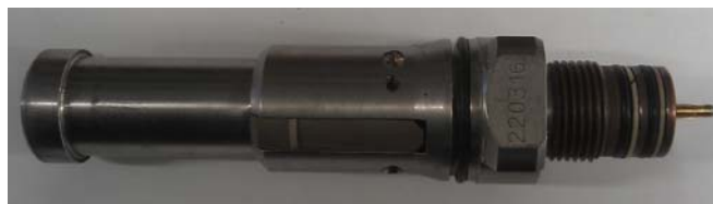
Figure 5-32 The Fishing Neck with Dog Latchings fitted
