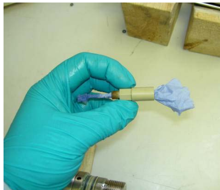
Figure 5-11 Clean the Lower Retaining Connector Nut
