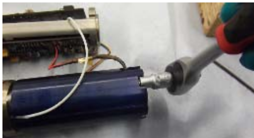
Figure 5-26 Remove the Hex Nuts with a Ratchet
