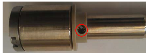
(Above) The Spool Feedthrough Mounting fitted and holes aligned
