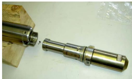
Figure 5-3 Removal of the Fishing Neck from the ADR
