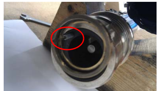
Figure 5-19 Alignment & fitment of the Soldered Conductor Ring
