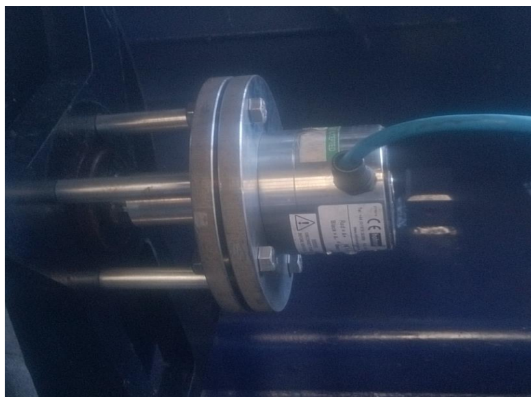
Figure 14 Install DTR encoder to ASEP wireline unit
