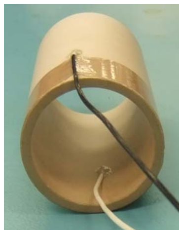
Figure 5-11 Tx Crystal Bonded Wire positions
