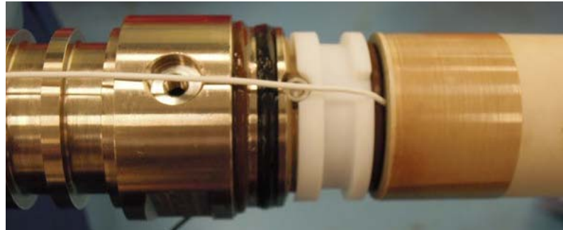
Figure 5-12 Tx Crystal Alignment on Tx Short and Piston Mandrel
