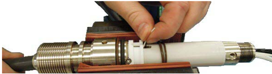
Figure 5-10 Tx Wiring through 'Transmitter' part of the Tx Short and Piston Mandrel
