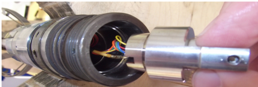
Figure 5.9 The LEMO Connector Assembly
