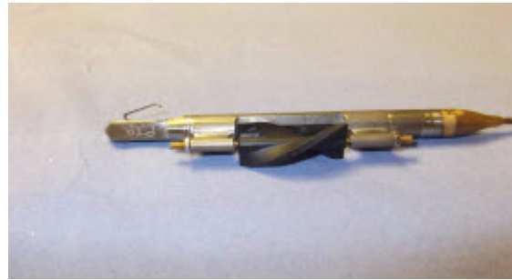
Figure 5.21 Spinner Assembly with magnet positioned centrally on Housing Assembly
