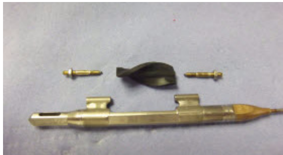
Figure 5.20 Removing the Nut from the Pivot Assembly
