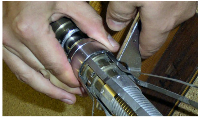
Figure 5.3 Sliding lower bow clamp ring away
