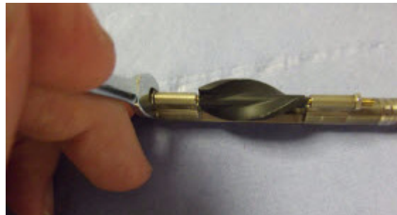
Figure 5.18 Loosening the Locking Nut
