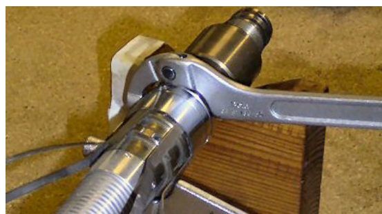
Figure 5.2 Loosen Bow Clamp Locking Rings
