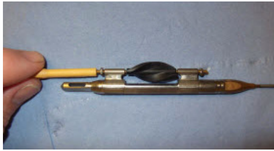
Figure 5.19 Unscrewing the Pivot Assembly with a Trim Tool
