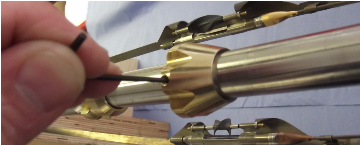
Figure 5.24 Fit Grub Screws into the Mounting Sensor Collar
