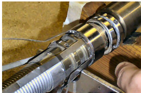
Figure 5.4 Loosening Bow Clamp Split Rings
