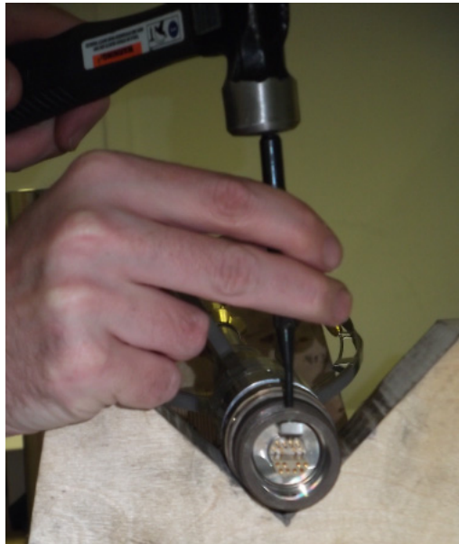
Figure 5.8 Removing the Spirol™ Pin
