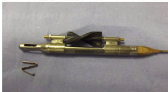
Figure 5.14 Sensor Assembly with Z-spring
