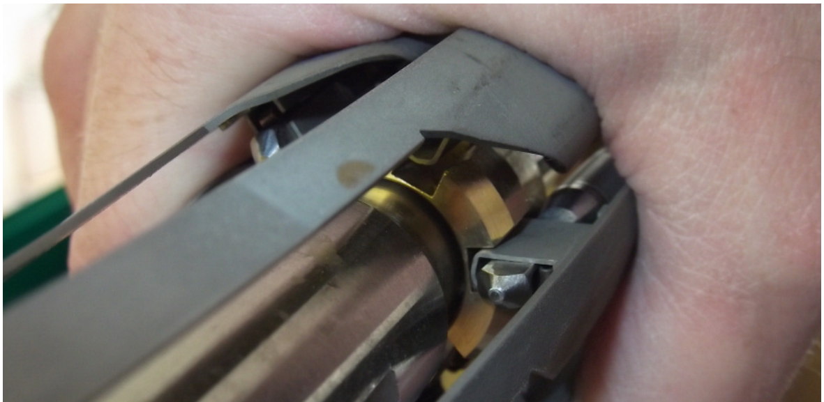
Figure 5.25 The Springbows nesting into the recesses of the Sensor Guide and Closing Collar
