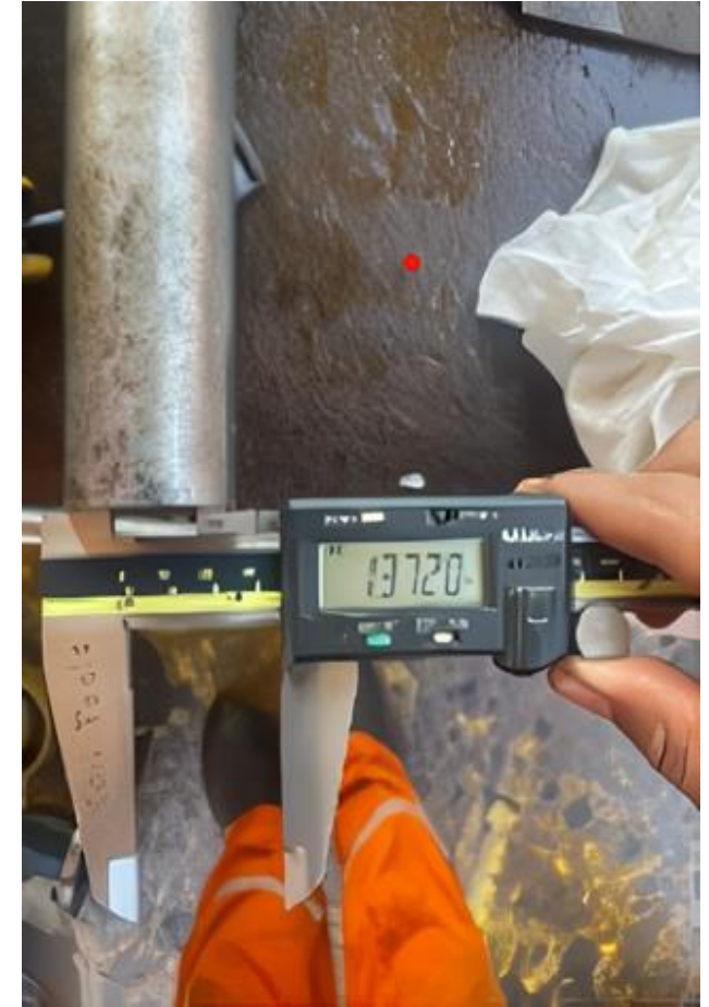
Figure 3 – ID of Packing mandrel = 1.372"
