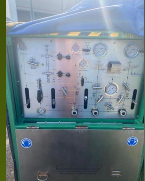
Well Control Panel
