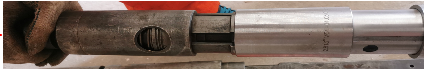
Fig 2 : GS Pulling Tool with Lock Mandrel
