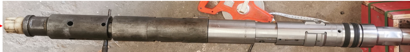
Fig 3 : X-Line Running Tool with Lock Mandrel
