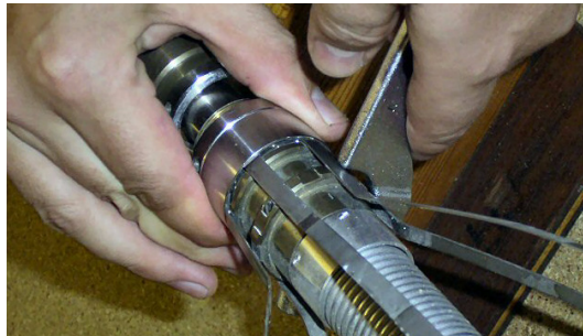
Figure 5.3 Sliding lower bow clamp ring away.
