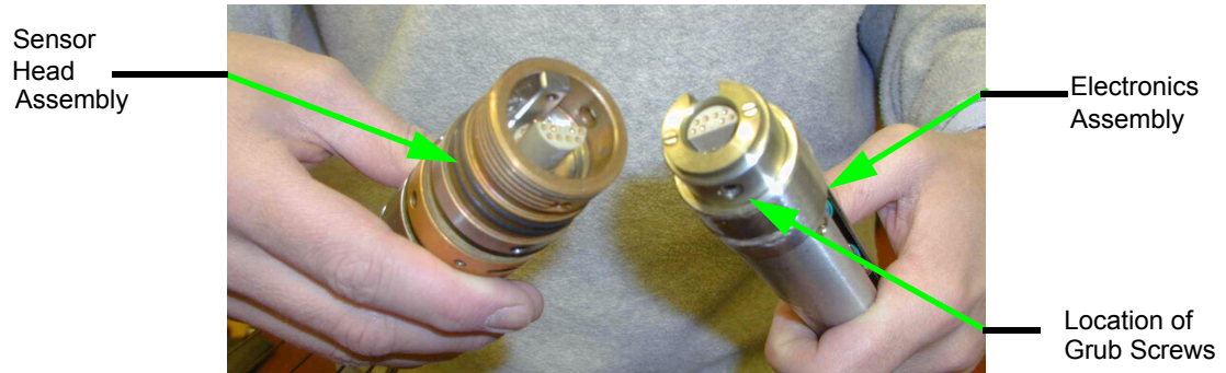
Figure 5.12 Connecting Electronics to Sensor Head
