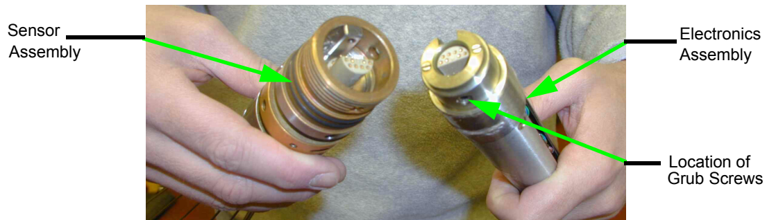
Figure 5.1 Separating Electronics from Sensor Head Assembly
