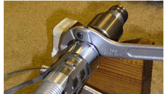
Figure 5.2 Loosen Bow Clamp Locking Rings
