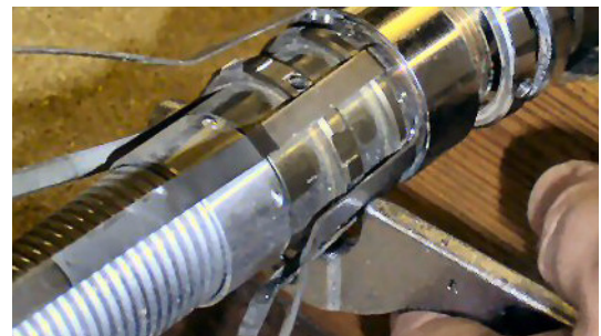
Figure 5.4 Loosening Bow Clamp Split Rings
