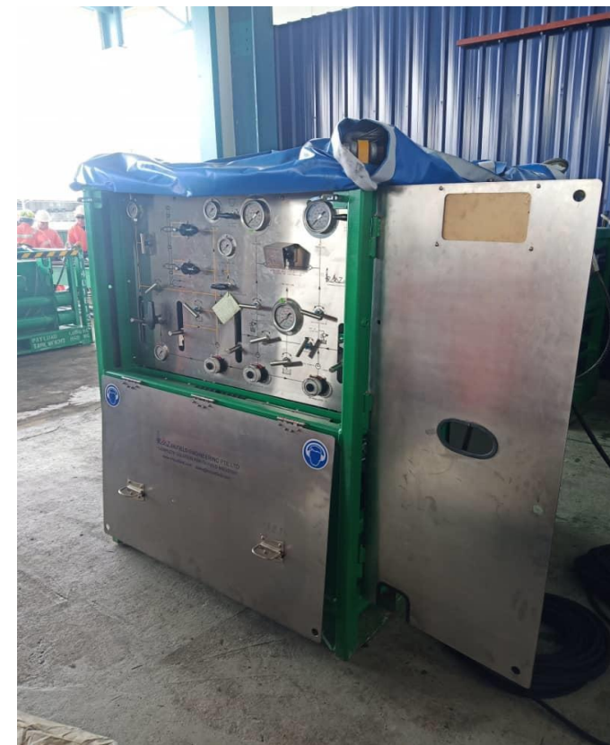
WELL CONTROL PANEL (WCP)
