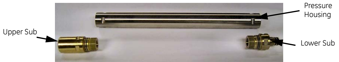
Figure 5-14 End Subs removed
