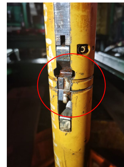
Image 2: Tubing cutter retain with single wire prior to RIH
