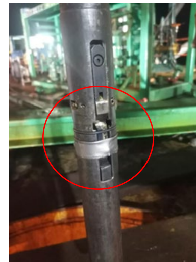
Image 1: Tubing cutter retain with O-ring & wrapped prior to RIH
