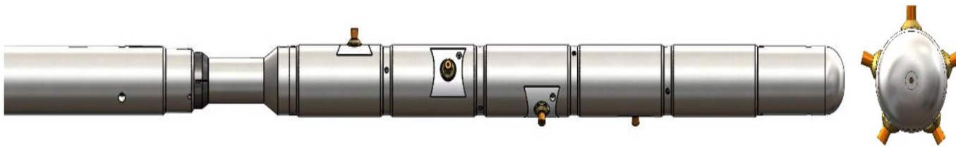
Figure 56 - Image showing 5 Punch Heads phased at 72°
