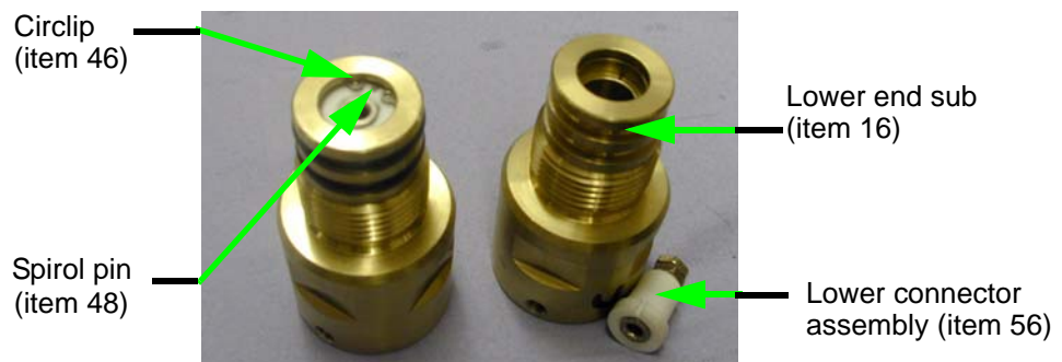
Figure 5.8 Removing Lower Connector Assembly
