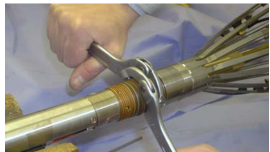
Figure 5.15 Tightening/loosening Bow Clamp Split Rings (tightening shown)
