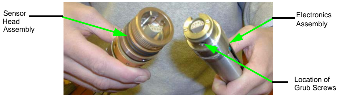
Figure 5.1 Separating Electronics and Sensor Assemblies
