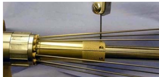
Figure 5.5 Slackening Grub Screws
