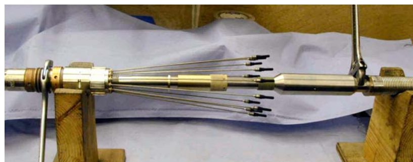
Figure 5.12 Tightening Central Shaft and Sensor Head
