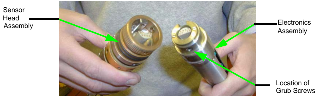
Figure 5.18 Connecting Electronics to Sensor Head
