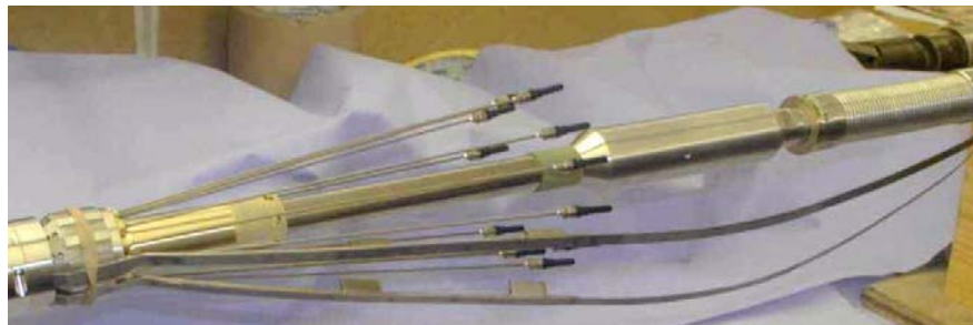
Figure 5.17 Fitting Springbow Assemblies
