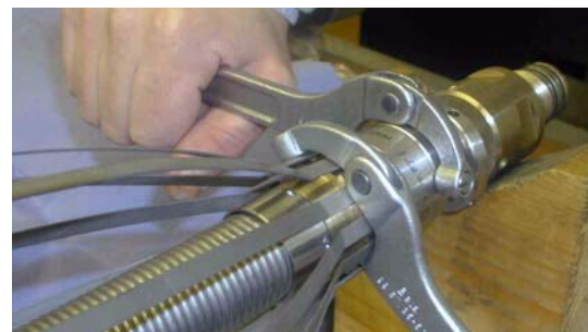
Figure 5.3 Using 'C' spanners to tighten/loosen Bow Clamp Locking Rings (tightening shown)
