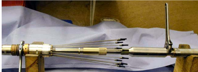
Figure 5.6 Unscrewing/tightening Central Shaft and Sensor Head (shown ready for tightening)
