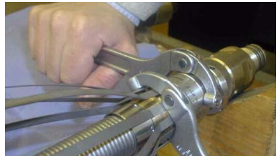
Figure 5.14 Tighten Bow Clamp Locking Rings
