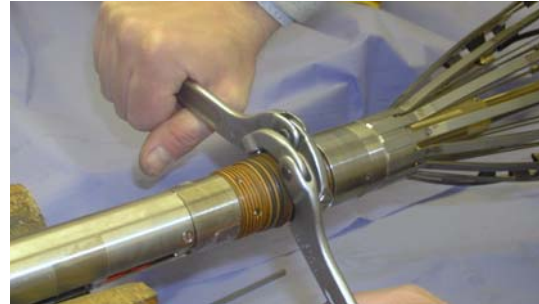
Figure 5.4 Tightening/loosening Bow Clamp Split Rings (tightening shown)
